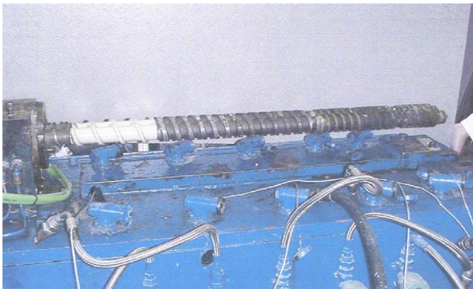
Figure 1: 40mm twin screw pulping unit at Brunel University UK showing internal shafts
