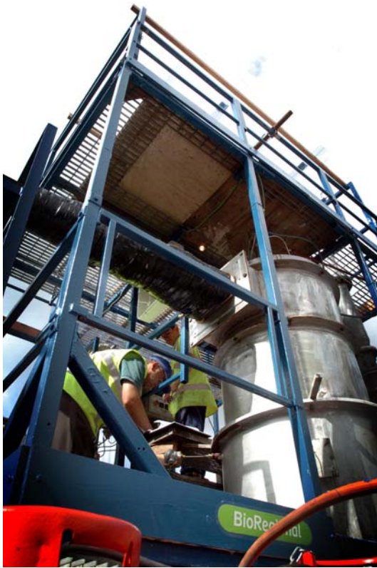
Figure 7 - Pilot scale black liquor chemical and energy recovery process being tested in Manchester, UK in 2006
